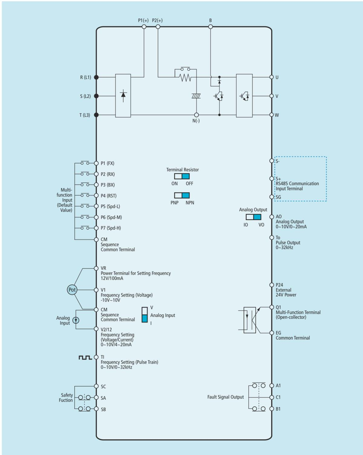
Standard Connection Diagram [30~75kW]
